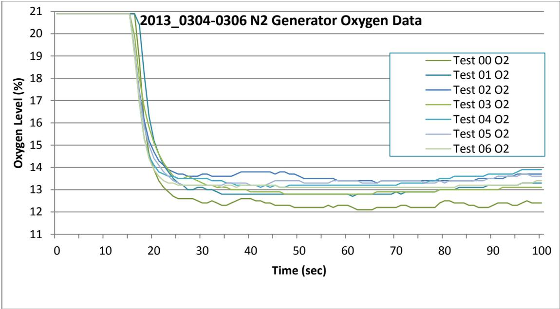
Chart G4: Graph showing an overlay of the oxygen level inside the test chamber after activation of one 2"x14" N2 generator from all seven tests.
