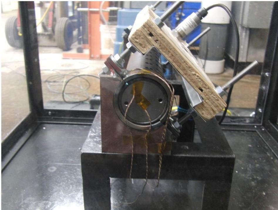
Photograph 8: Blank end view of the test fixture, showing the placement of the thermocouples and 1 inch separation distance.
