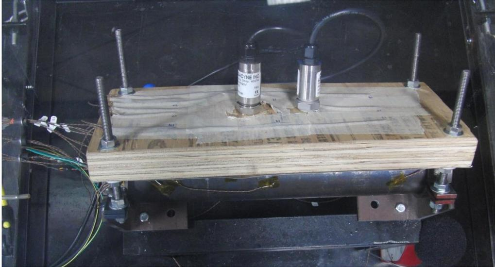
Photograph 9: Top view of the test fixture showing the installation of both pressure transducers for Test 04.
