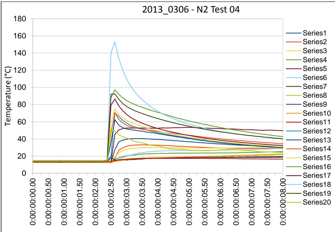
Chart T10: Temperature profile of the heat transfer panel during Test 04.fg
