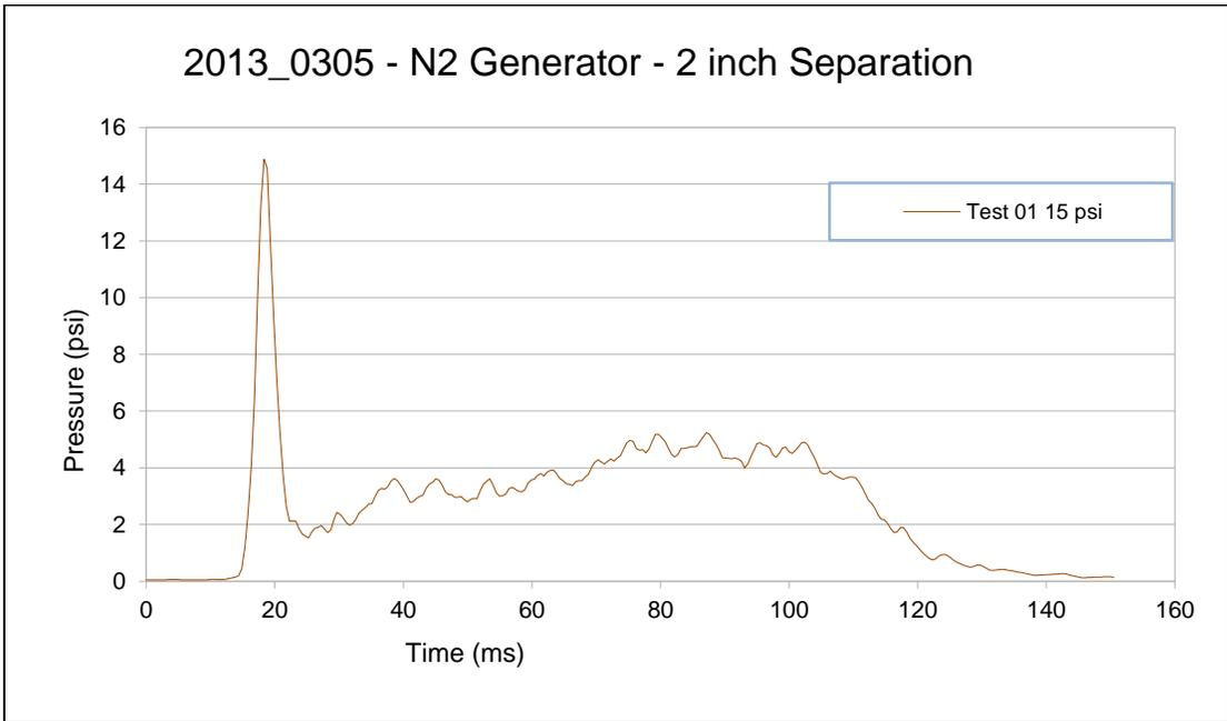
Chart 3: Graph showing the pressure recorded from the 15 psi transducer at 2 inches from the generator.
