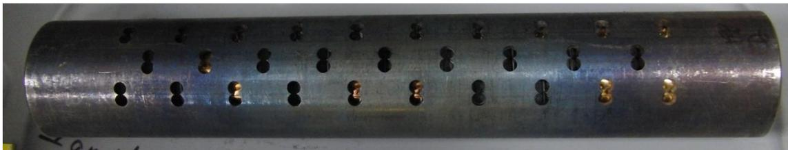
Photograph 11: Photo showing typical burst foil removal ratio of 70% for the 0.004" thick burst foil. Subsequent testing will be performed with 0.002" material.
