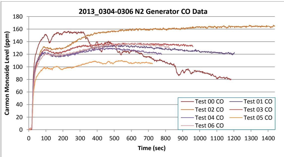
Chart G3: Graph showing an overlay of the carbon monoxide levels inside the test chamber after activation of one 2"x14" N2 generator from all seven tests.
