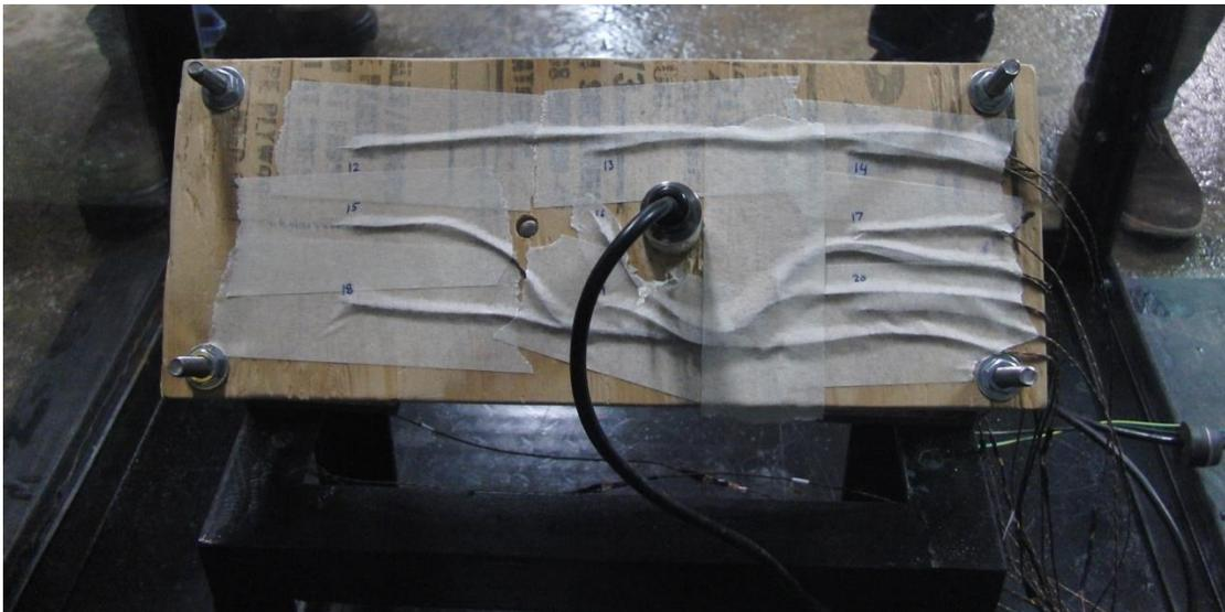
Photograph 6: Photo of the outside of the backing plate. The arrangement of the thermocouples and the single pressure transducer can be seen.
