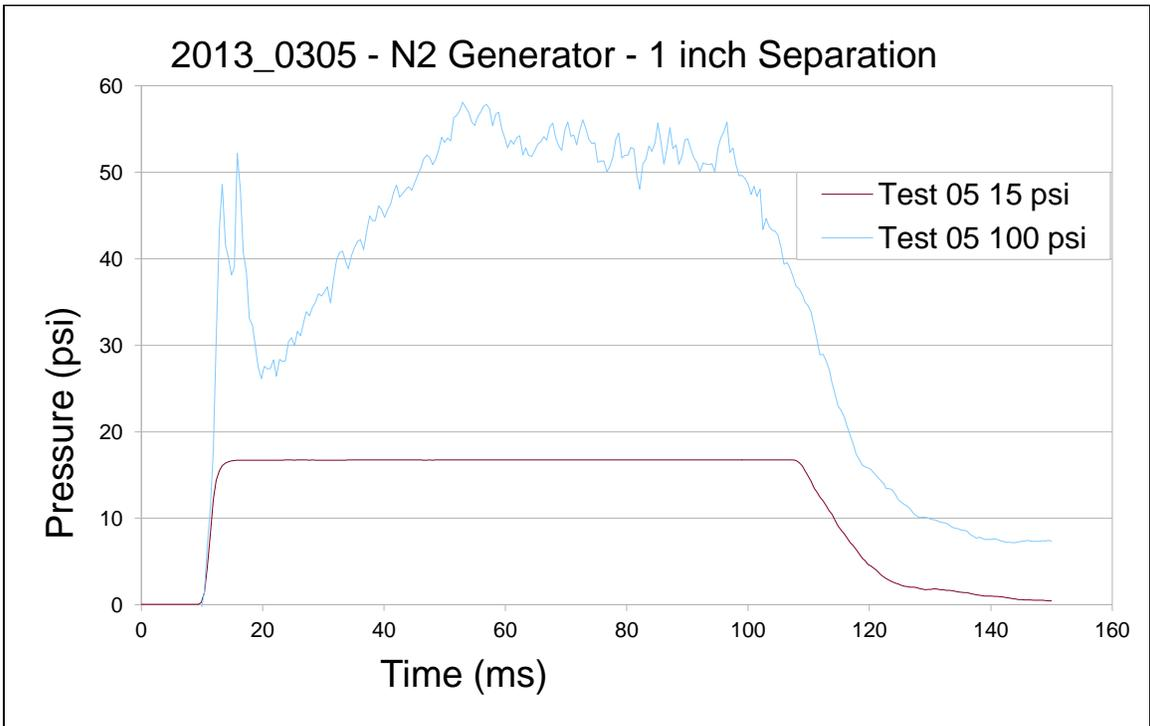
Chart 7: Graph showing the pressure traces recorded at 1 inch from the generator during Test 05. The 15 psi transducer clipped during the bulk of the event.
