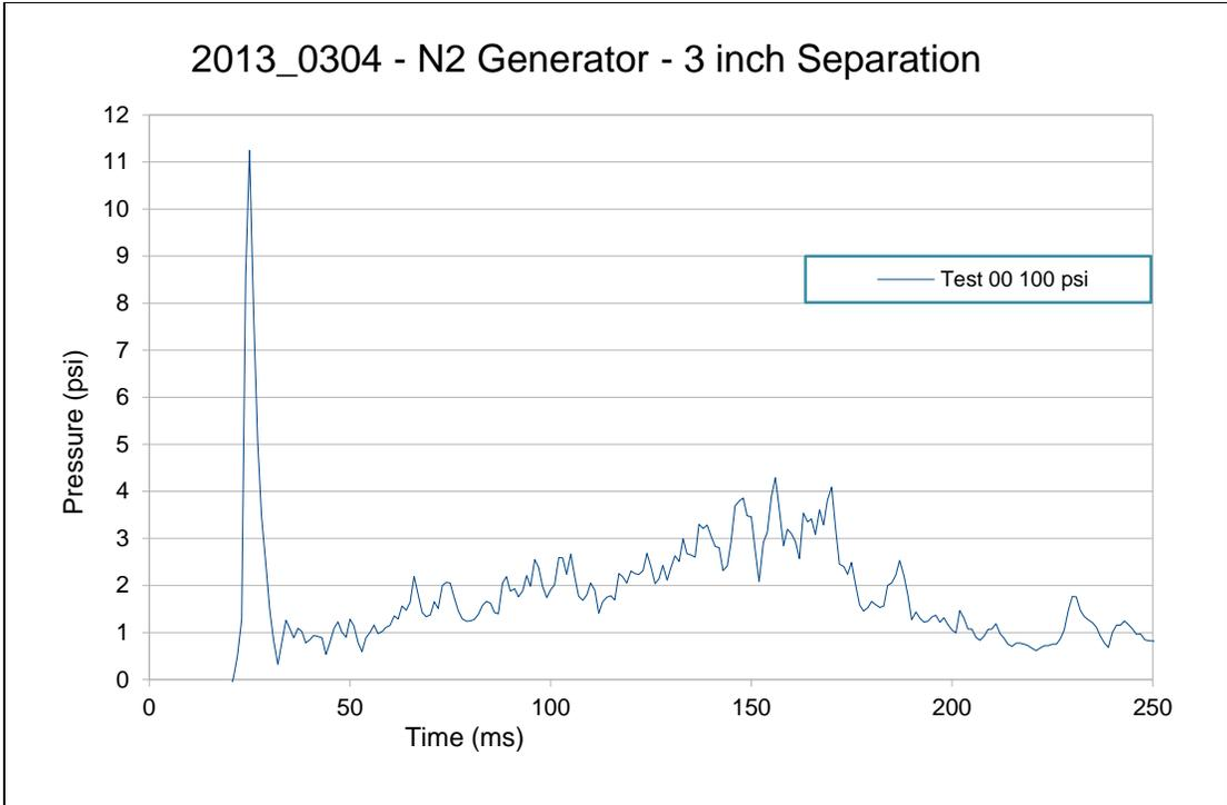
Chart 2: Graph showing the pressure recorded from the 100 psi transducer at 3 inches from the generator.
