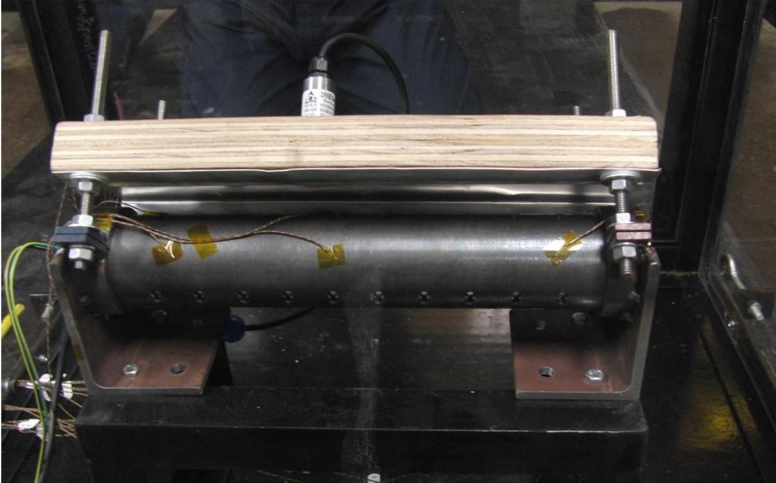
Photograph 5: View from the front of the test fixture, showing the arrangement of the thermocouples attached to the generator body. The igniter end of the generator is towards the left side of the photo.
