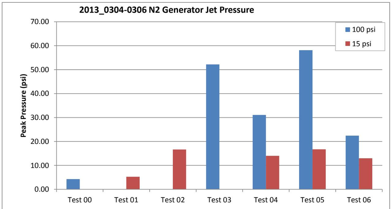
Chart 1: Graph showing the relative jet pressures recorded and the spike attributed to electrical noise at the beginning of the test.
