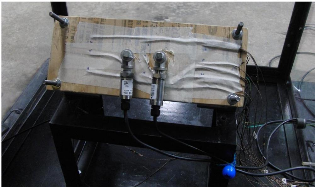
Photograph 10: Rear view of the test fixture showing the installation of both pressure transducers into the tees for Tests 5 and 6.
