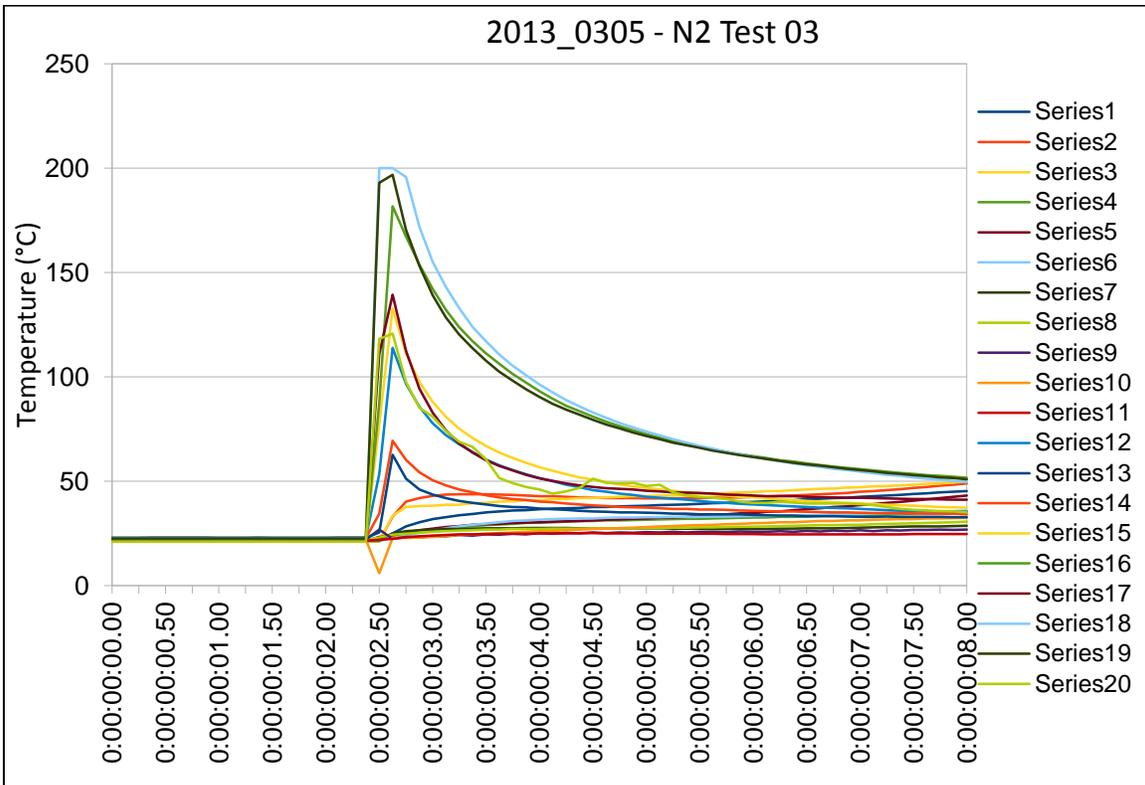
Chart T8: Temperature profile of the heat transfer panel during Test 03.
