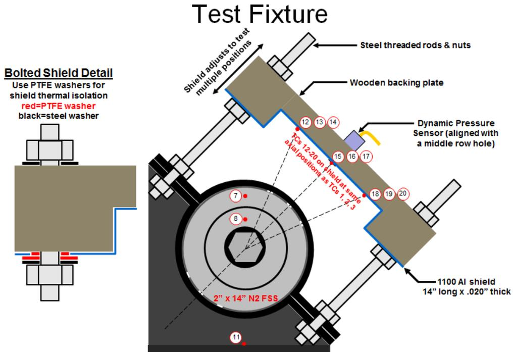
Figure 3: Drawing supplied by Boeing engineers showing the test fixture construction and thermocouple placement (#12-#20).
