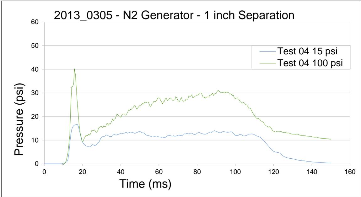
Chart 6: Graph showing the pressure traces recorded at 1 inch from the generator during Test 04.
