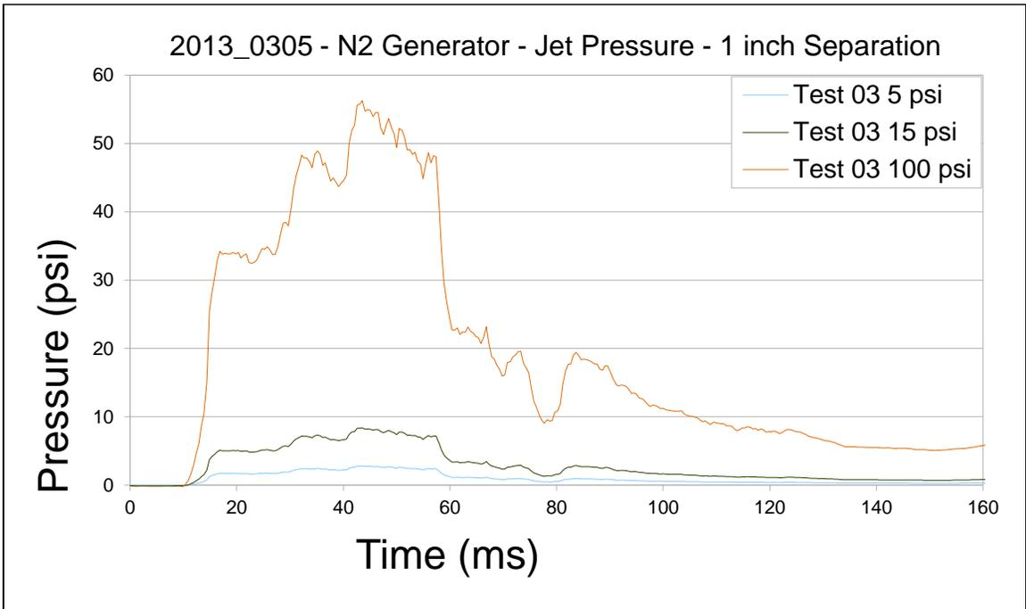
Chart 5: Graph showing the pressure traces recorded at 1 inch from the generator during Test 03. The trace from the 100 psi transducer was the proper channel, the 5 psi channel was mistakenly reported immediately after the test.
