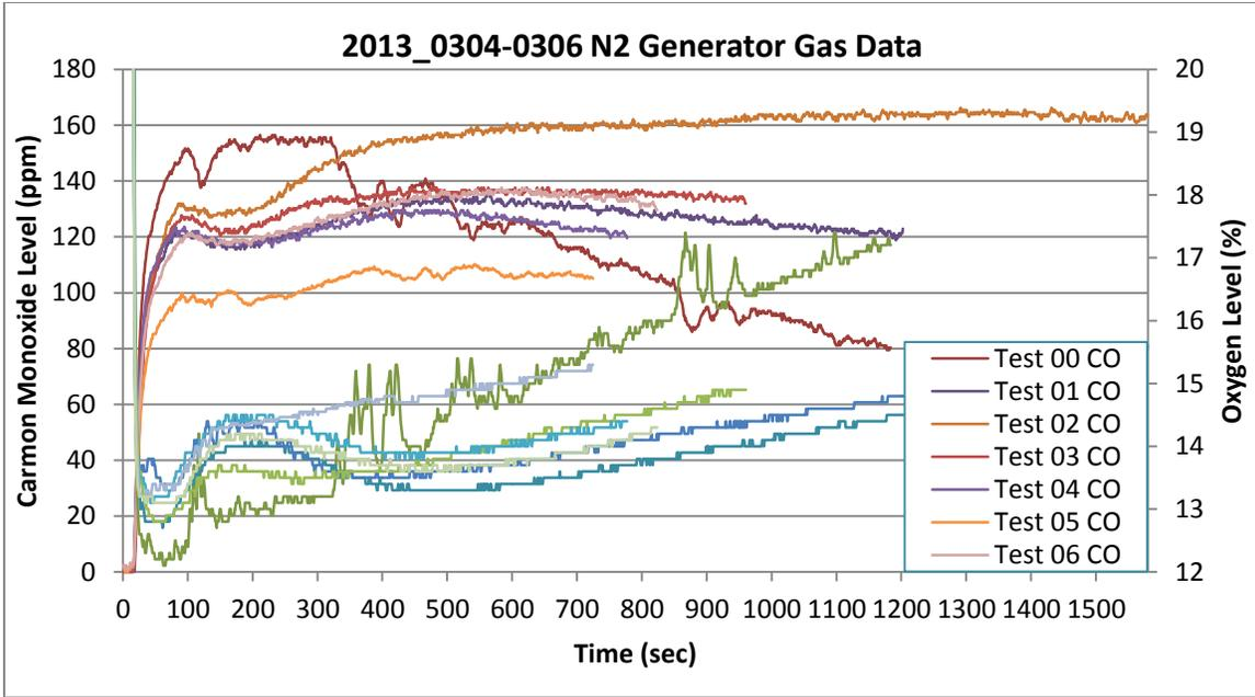
Chart G2: Graph showing an overlay of the oxygen and carbon monoxide levels from all seven tests.
