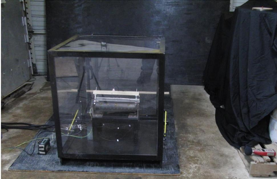
Photograph 1: Photograph of the test setup. The test chamber can be seen in the center of the photo. The sound level meter is located in the lower right corner of the photograph as placed in Test 01. The test fixture can be seen mounted inside the center of the test chamber. The gas monitor can be seen just to the left of the chamber.
