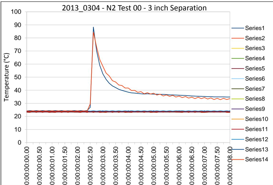
Chart T2: Temperature profile of the heat transfer panel during Test 00.
