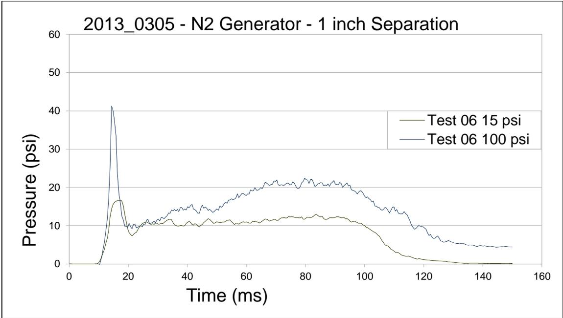
Chart 8: Graph showing the pressure traces recorded at 1 inch from the generator during Test 06.
