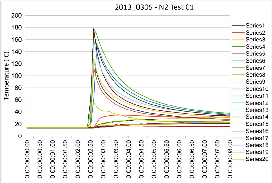
Chart T4: Temperature profile of the heat transfer panel during Test 01.
